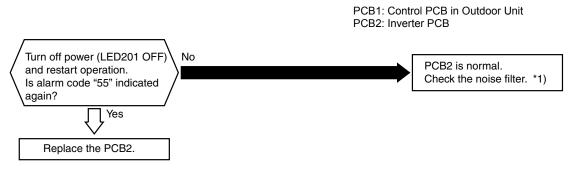
\*1): When the unit is applied the excessive surge current due to lightning or other causes, alarm code "55" or Inverter stoppage code (IT) "11" is indicated and the unit cannot be operated. In this case, check to ensure the surge absorver (SA) in the noise filter (NF1, NF2). The surge absorver may be damaged if the inner surface of the SA is black. If so, replace the surge absorver.
